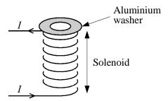
A large direct current is switched on in the solenoid. Explain why the washer jumps and immediately falls back.
